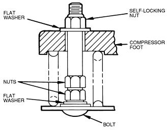
Fig. 12 — Compressor Mounting
